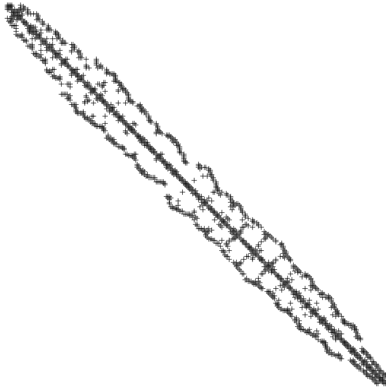
Figure 3: Sparsity of the FE Matrix After Renumbering
