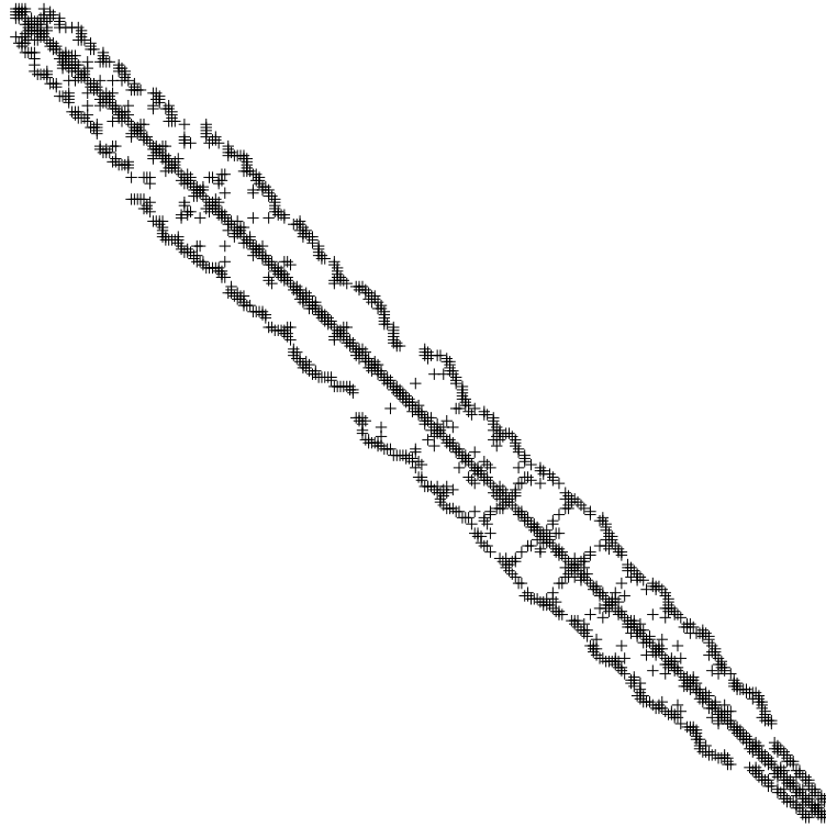
Figure 3: Sparsity of the FE Matrix After Renumbering
