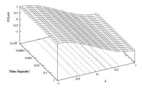
Solution, U(2,x,t), of Elliptic-parabolic Pair using Chebyshev Collocation and BDF
