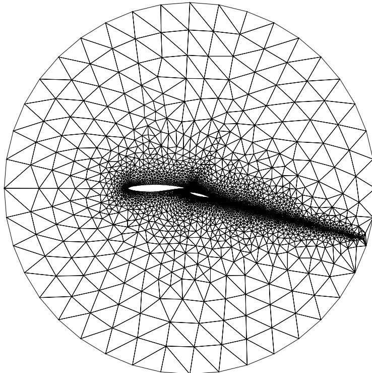
Mesh Generated Using Geometric Coefficient  $\omega=1.0$
