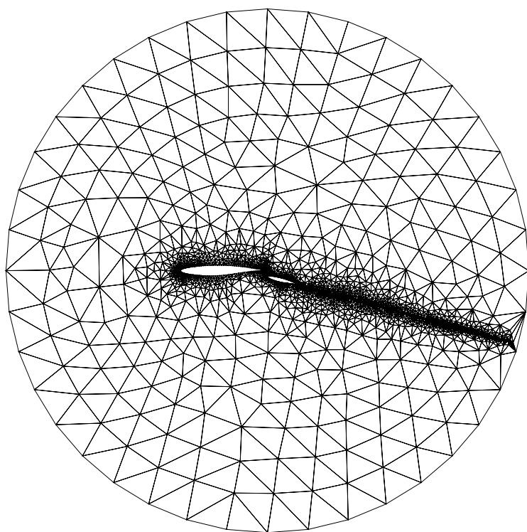
Mesh Generated Using Arithmetic Coefficient  $\omega=1.0$
