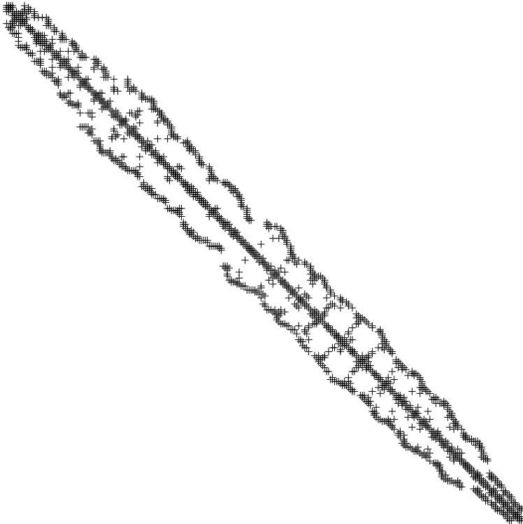
Figure 3: Sparsity of the FE Matrix After Renumbering
